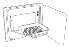
The Handyrack fits to the left hand oven door only. Food cooking on it is easy to attend to, because it's accessible when the door is open. It can be fitted at two different heights. One of the oven shelves must be removed and the other positioned to suit.
